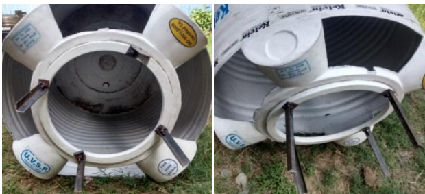
Figure 2: Agitator fitted in tank
