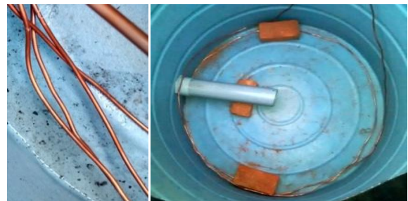
Figure 4: Copper tube fitted in tank
