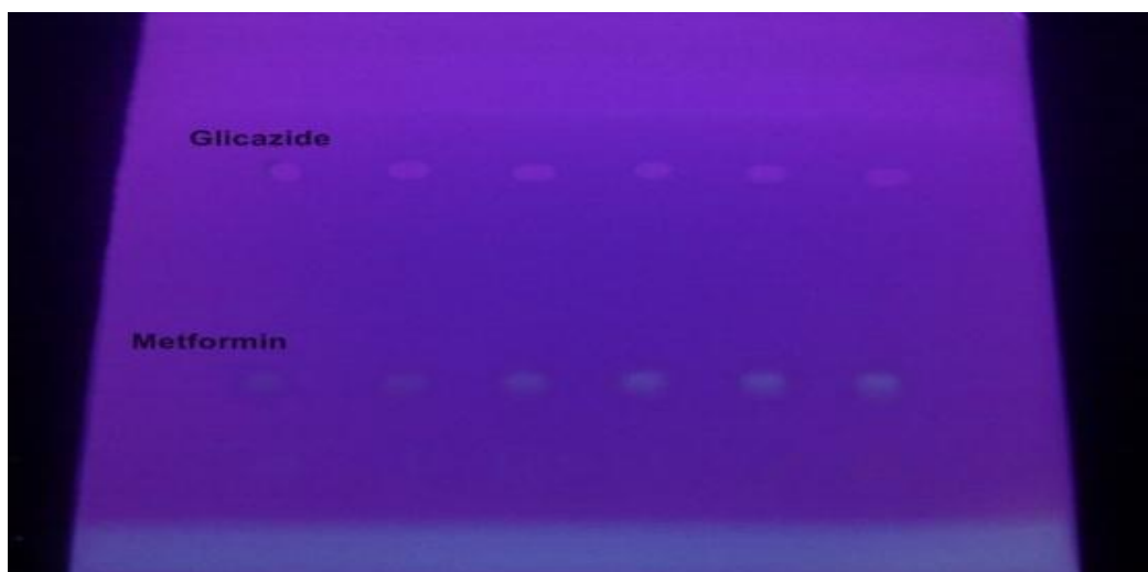
Figure 3: TLC Plate showing separation of (GLZ Rf =0.67) and MET (Rf =0.39)
