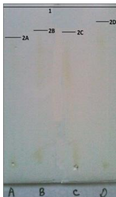
Figure 1: TLC profile of test solution of all three marketed formulations and in-house formulation. 1- Distance traveled by solvent, 2 - Distance traveled by solute. A- Dabur ashokarishta, B- Sandu ashokarishta, C- Baidhyanath ashokarishta, D- In-house formulation
